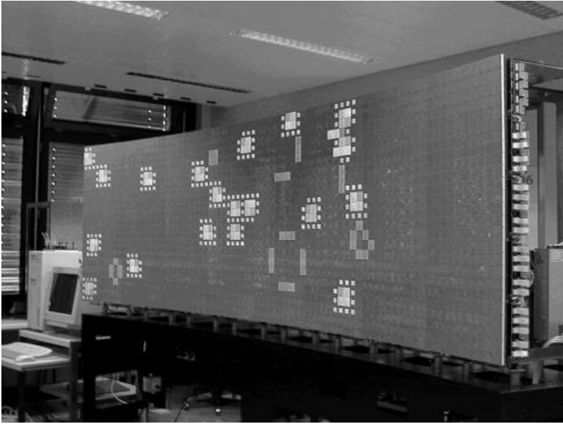
Fig. 7. The BioWall used to physically implement our Life/loop CA. The dots surrounding the loops define visually the loop context (Photograph by A. Badertscher).
